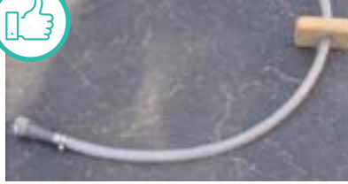
Hose has no kinks and includes a sponge to reduce leakage at penetration when insulating. Courtesy of South Seattle Community College
