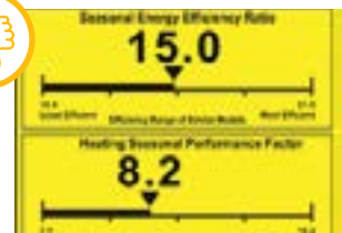
HSPF is below 9.0 specification.
